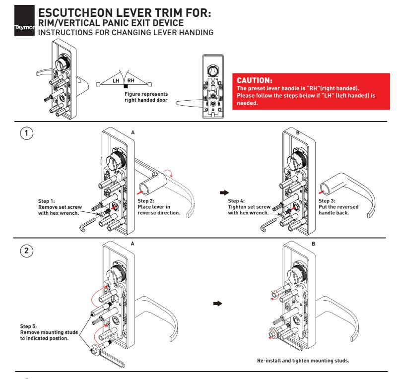
**3** The setting for switching handle direction is completed.
