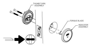
Insert torque blade horizontally into deadbolt latch. Crank until indicator assembly is flush with the door face. Mate the thumbturn assembly with the torque blade on the indicator assembly. Insert the screws through the holes of the thumbturn assembly and latch body. Tighten the screws to the threaded posts of the blank mounting plate. Tighten the assembly so the complete assembly is tight to the door.
