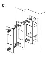
Match screw holes on strike with vertical center lines on jamb. Mark outline of strike and chisel 1/4" (6.4 mm) deep for flush fit of dust box, wood frame reinforcer, and strike. Place dust box and wood frame reinforcer into mortise area ad tighten to the frame using 3" wood screws. Insert the strike and tighten to the frame with #8 screws.
